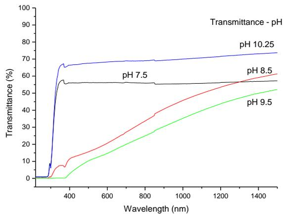
**Fig.3(b) Transmittance spectra of ZnO nanorods with different pH**
