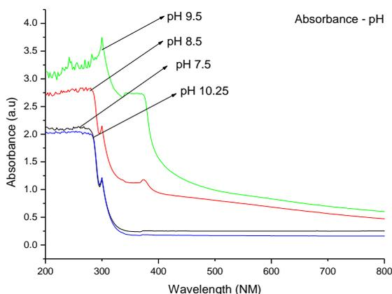
**Fig.3(a) Absorption spectra of ZnO nanorods with different pH**
